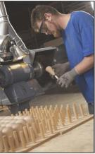
Approximately 90 percent of the sanding is done by the robot. Shift knobs are given quick touch ups and are inspected for quality.
