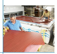
This year, Paladin is completing a \$2 million investment in WMIA machinery for a one-piece-flow solution in its membrane press work cell to contend with offshore competitors in office system components and store fixture markets. The company's goals are to eliminate as much material handling as possible, increase throughput production flexibility and lower labor costs.
