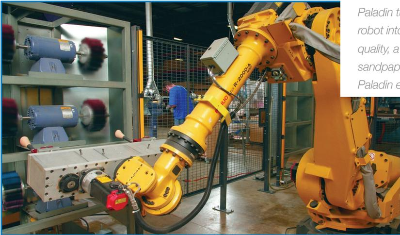
*Paladin turned to a WMIA member company to install a six-axis robot into its sanding work cell. In addition to consistent sanding quality, a 50-percent labor savings and substantially lower sandpaper costs, the investment also paid off by helping Paladin earn its customer's business for another four years.*
